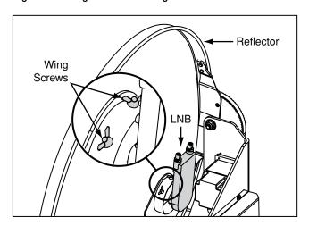
Figure 28: LNB Skew Angle Adjustment
